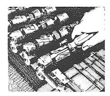
**3.** Then if required, remaining build-up can easily be removed by slight scraping.
