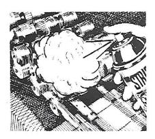
Spray The Stripper at those points where galvanizing tends to build up on your machines. The special cleaning ingredients get right to work softening up deposits.
